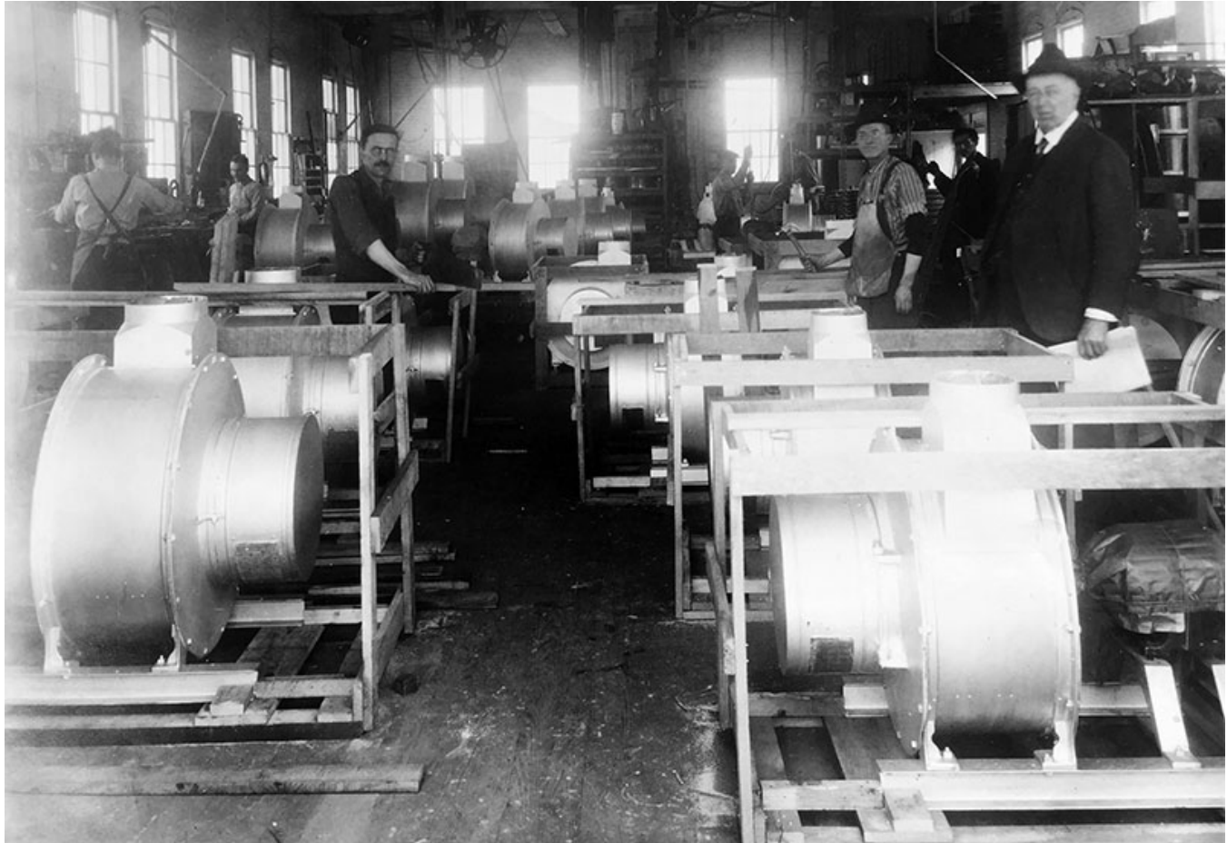
Figure 7: Schantz Organ Company, interior view of the Zephyr Organ Blower manufacturing space, undated. Courtesy of Schantz Organ company archive.
